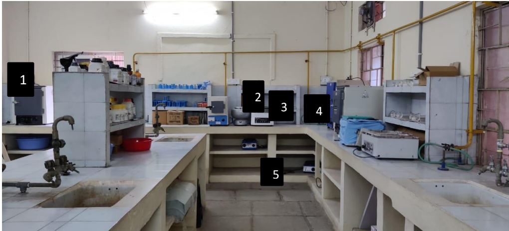
1. Hot Air Oven 2. Muffle Furnace 3. Desk Top Centrifuge 4. Haematocrit Centrifuge 5. Hot plate
